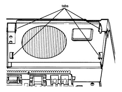
Lift up the subassembly from your work surface and lower the back end into the computer, guiding the top slots on the subassembly into the top tabs on the computer.
